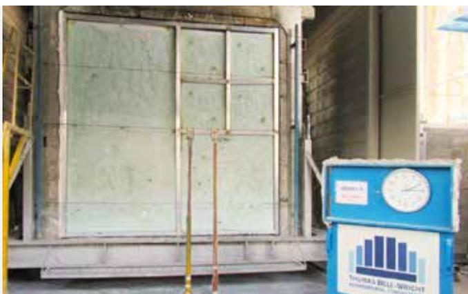
The picture presents the specimen view after the 120 minutes test where performed. The photo was taken on the unexposed side.
