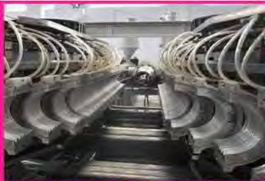
Pipe making line Extrusion line for double wall corrugated pipe
