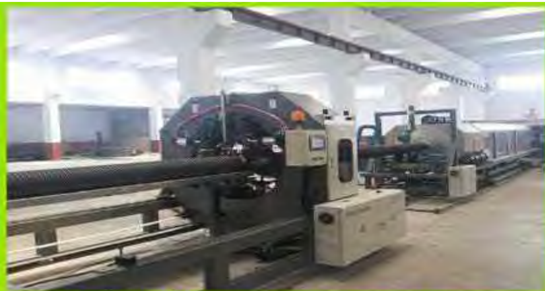
Extrusion machine for Double wall corrugated pipe
