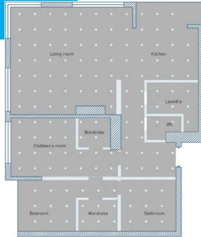
■ Frame soundproofing ceiling on ULTRAKUSTIK hangs (130 mm)
