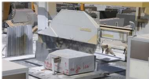
Disk Machine for trimming of Blocks & Sawing of big Thickness.
