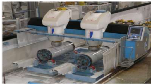
Polishing Machine of Curved Surfaces as columns.
