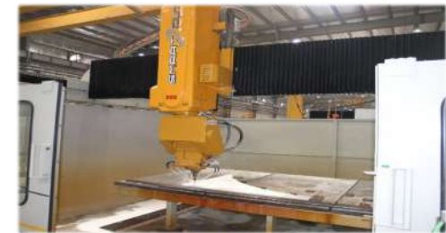
Smart Cut Machine for Engraving of Arches.
