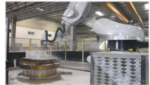
Robot Machine for Carving of Column Capitals, Muqarnas and decorative Items.
