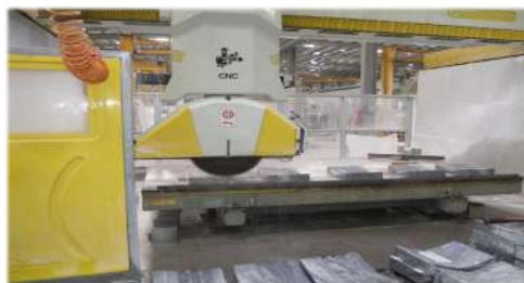
CNC Machine for Profiling Curved items (3D) as SOFFITS etc.
