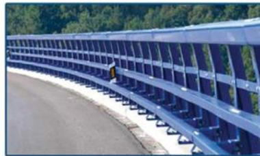
HIASA manufactures, supplies and installs metallic bridge-vehicle parapets with different Containment levels: High (H2, H3) and Very High Containment (H4b), called "PMH-13", "PMH-16" and "PMH-38", respectively. These metallic safety barriers have been specially designed for bridge deck sides (bridges, viaducts, etc.), the top section of retaining walls and other similar works.
