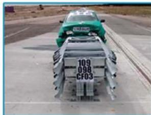
The "AIR" redirective crash cushions are fully manufactured with galvanized steel and have a compact, open and exposed design that is easy to inspect.
